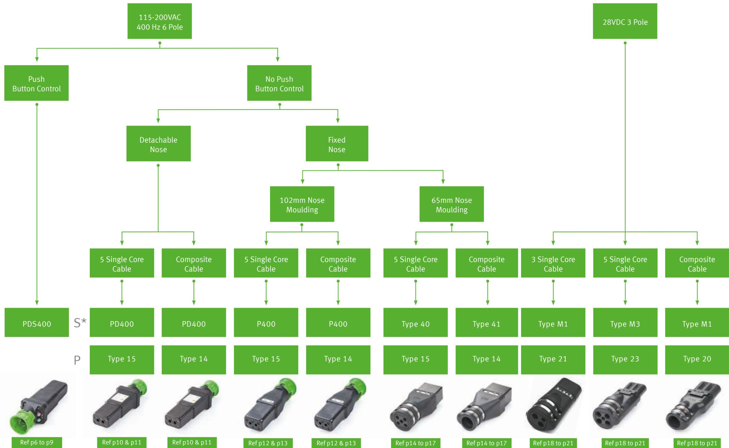
\* S - Sockets (plug into the aircraft - have tubes)
